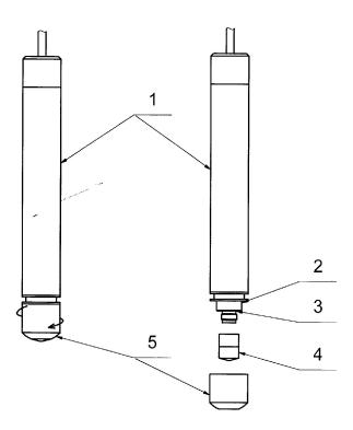
Fig. 1 Sensor CSOT 63-88 - exchange of membrane head
