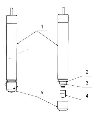
Fig. 1 Sensor CSOT 63-66 - exchange of membrane head
