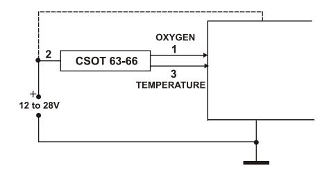
Fig. 2 Sensor connection to external device
