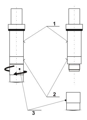
Fig. 1 Sensor CSOT 53 - exchange of membrane head
